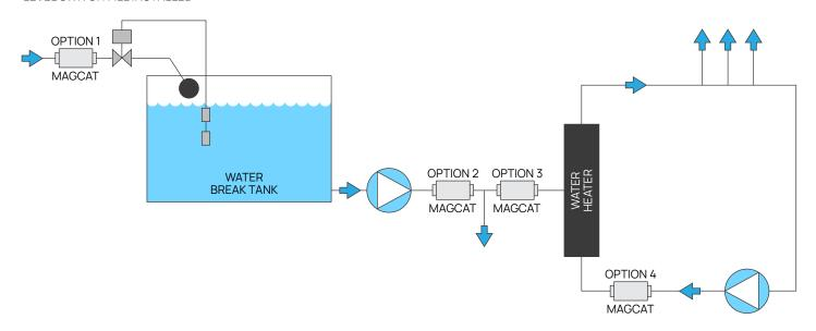
A water conditioning device induces nucleation of hardness scale and in doing so prevents hard deposits forming. As such, a water conditioning device does not remove the hardness and may still be present in evaporative conditions.
