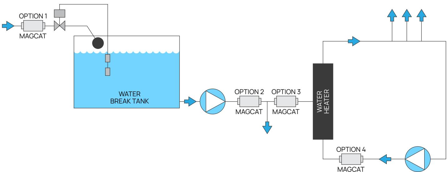
A water conditioning device induces nucleation of hardness scale and in doing so prevents hard deposits forming. As such, a water conditioning device does not remove the hardness and may still be present in evaporative conditions
