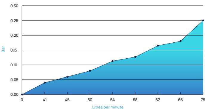
Both our catalytic and combination (dual) systems have internal components designed specifically to minimise resistance as water passes through
